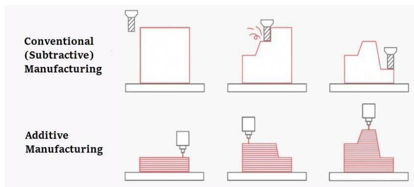
Attaran [5] identifies five key benefits that AM has over traditional manufacturing: Cost, speed, quality, innovation, and impact. Manufacturing processes between CM and AM are different in the nature and approach. As shown in Figure 1, CNC machining, one of the most common CM technology, typically subtracts a solid block of material to achieve the final shape, while AM proceeds in an additive manner, adding material one layer at a time.
